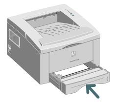
Insert the tray back into the printer.
